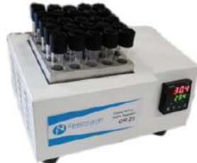
Closed Reflux Digestor
