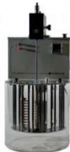
Water separability of petroleum oils and synthetic fluids
